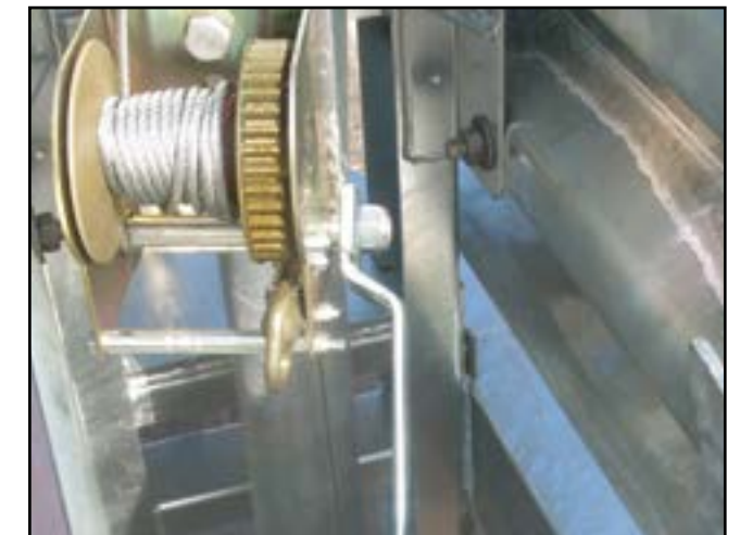
Figure 5 - Winch attached to the Anchoring picket
