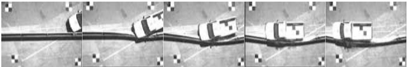
For all tests above the vehicles where safely re-directed by the **Orion**<sup>™</sup> barrier. The vehicles did not penetrate, underride or override the test installations. The test article was judged to have satisfied the requirements of NCHRP Report 350 criteria TL-3 for a longitudinal barrier.
