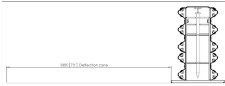
**Note:** Results are from actual crash testing and the test article length was 70m (230'). Results from Test 3-11 (NCHRP 350) are the published TL-3 Deflection.
