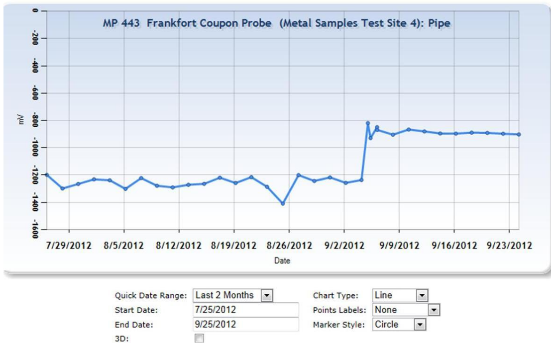
Figure 11 – Carrier pipe potential measurements (note “event” on 9/5/12)
