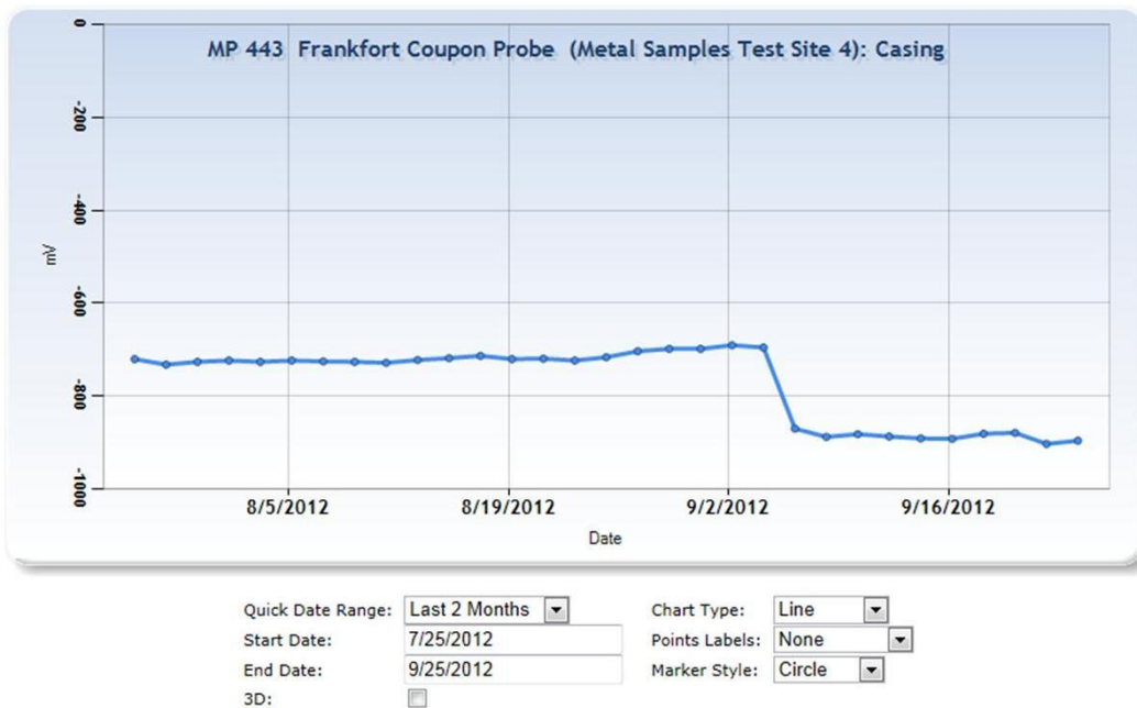
Figure 10 – Casing potential measurements (note “event” on 9/5/12).
