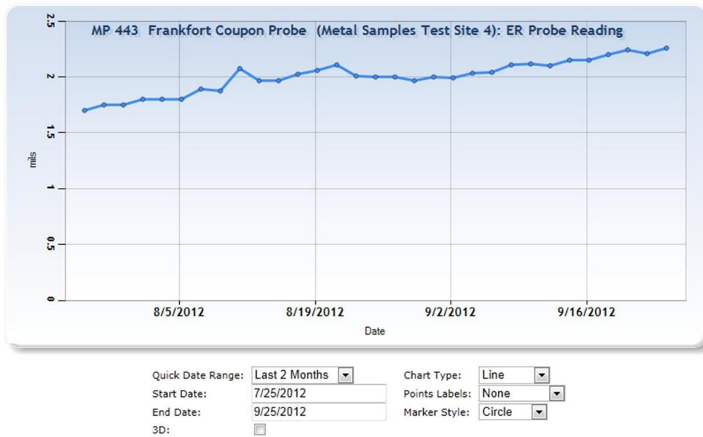
Figure 9 – Graphical display of corrosion rate in mils per year from test site (screen shot).
