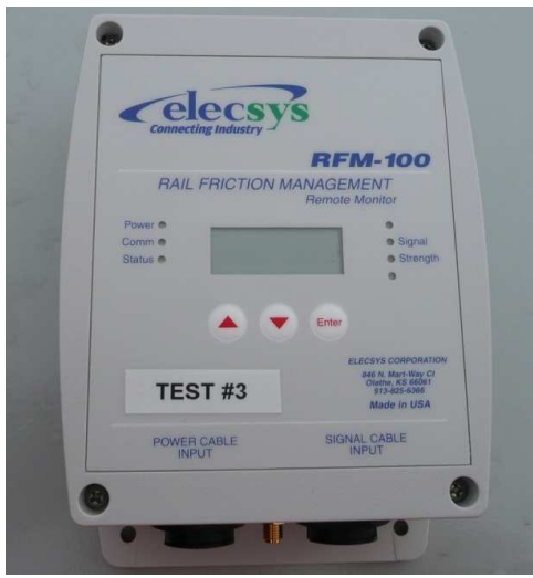
Figure 8: Remote Monitor Actual Size 5.4x7.8x2.8 inches (135x200x72 mm)
