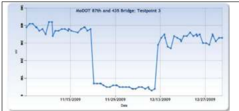
Figure 8: Graph of Zone 3 potential data points showing failure from November 22, 2009 to December 12, 2009
