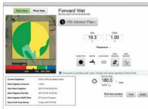
View current soil water depletion map and current pivot operational status, plus a summary of key actionable information with availability to directly select manual or VRI mode and control irrigation equipment.
