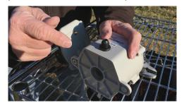
(For top of post mounting, prep the unit by feeding the cable through the hole in the top of post adapter, then using the screws, washers, and nuts provided secure the adapter to the unit.)
