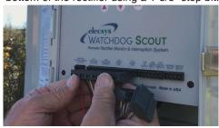
Step 3: Plug cable assemblies into Scout. Leave power cable unplugged until input voltage is confirmed at the end of installation
