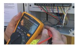
Step 12: Turn the rectifier on and check the voltage at the Scout power plug by touching the Meter leads to the connector screws on the plug. The voltage should be 12VAC to 14VAC.
