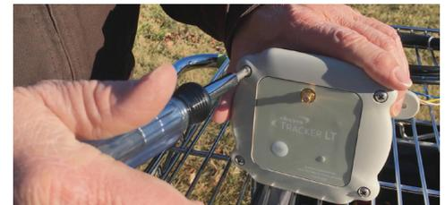
Step 2: Remove the 4 screws in the top of the unit to gain access inside and swap the cord grip and plug already in the unit.
