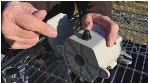
(For top of post mounting, prep the unit by feeding the cable through the hole in the top of post adapter, then using the screws, washers, and nuts provided secure the adapter to the unit.)
