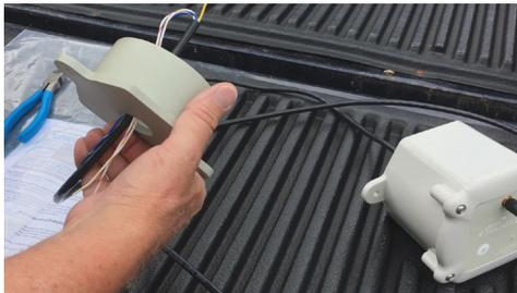
Step 1: Determine if the unit will be mounted on the top of the test point post or on the side of the post.
