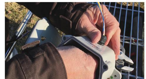
Step 3: Thread cabling through cord plug in the side of the unit.
