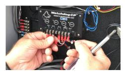
Step 3: Remove the wires from the Smart Node and the top right side of the terminal block on the lower left of the WD2 enclosure.
