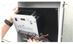
Step 7: Remove the four screws in the corners of the Back Panel and remove the back panel from the enclosure.
