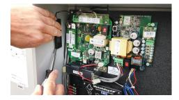
Step 4: Using a flat blade screwdriver remove the Hershey bar antenna from the top left side of the enclosure and unplug the GPS antenna from the Interrupter board.
