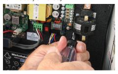
Step 6: Remove the screws holding the Mercury relay to the Back Panel and let the relay and wires lay to the outside of the enclosure.
