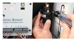
Step 9: Using the screws that were holding the relay to the old Back Panel, install the relay in the new Back Panel in the pilot holes to the right of the Scout unit made for that purpose.
