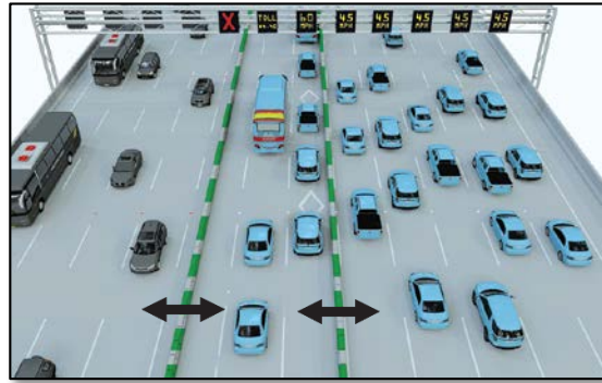
Moveable barriers allow flexibility for reconfiguration.
