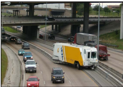
Contraflow lanes run on both sides of I-30 in Dallas, TX
