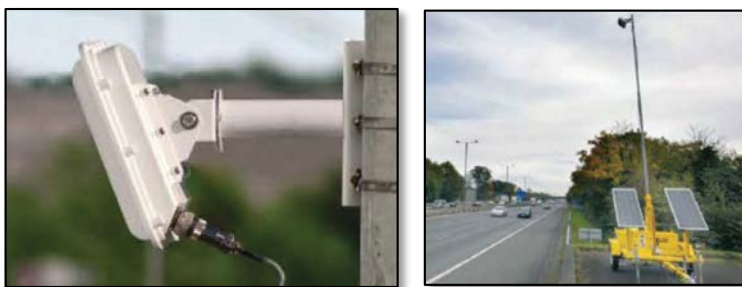
Solar powered microwave radar detectors gather real-time traffic data for DRUM
