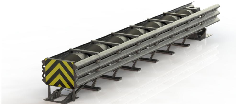
The Universal TAU-M™ Parallel, (TAU-M™) is a redirective, non-gating crash cushion. The TAU-M™ system has been tested and evaluated per the recommendations set forth in the Manual for Assessing Safety Hardware (MASH) Test Level 3 & Test Level 2. The TAU-M™ system utilizes tensioned cables, telescoping thrie-beam panels, and energy absorbing cartridges (EAC) to absorb kinetic energy and safely contain or redirect impacting vehicles.
