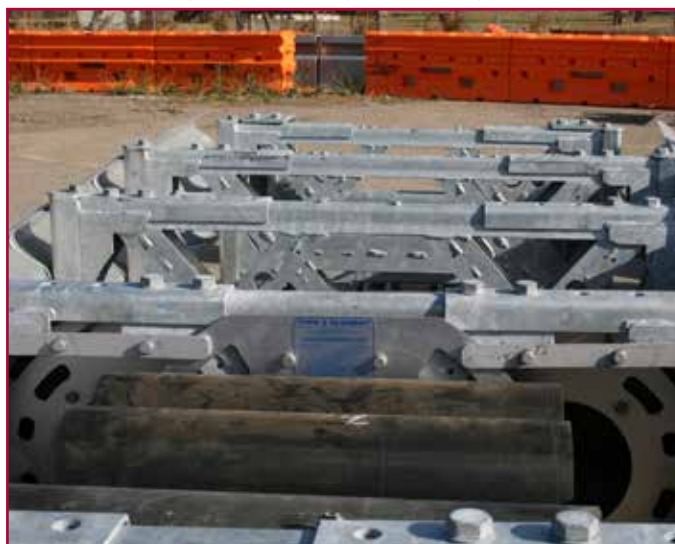
EAEs Secured with Mounting Brackets
