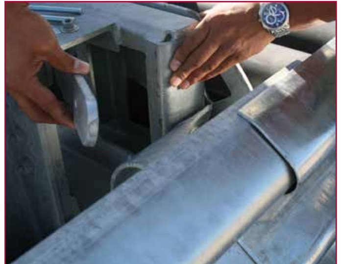
Mounting Bar used to Secure Element
