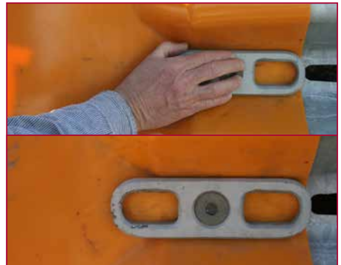
Installing Tow Hooks on Nose Cover
