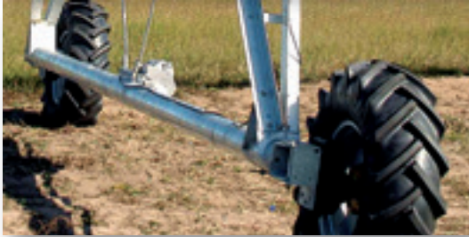
Advanced drive line (center drive and PowerDrive gearbox)
