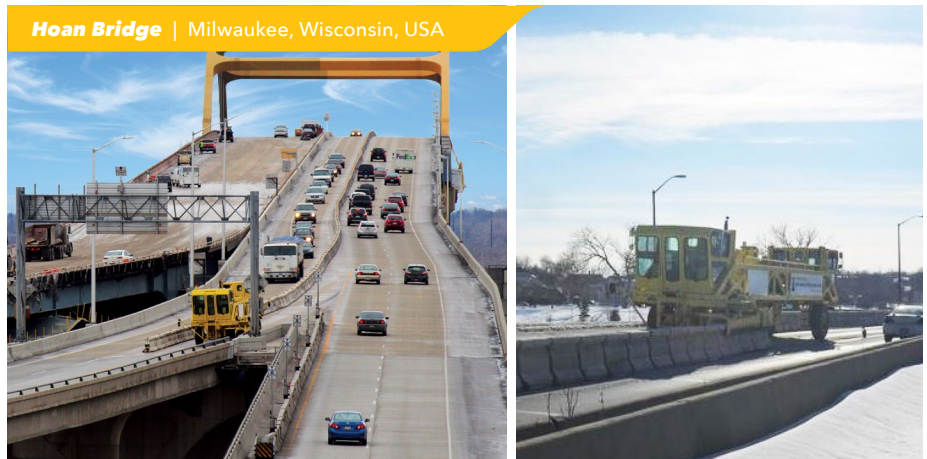
To mitigate traffic congestion, the Road Zipper reconfigures the roadway in real time to give two lanes to the peak travel lanes at all times.
