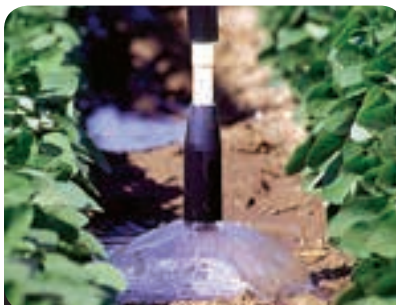
Low Energy Precision Application (LEPA) nozzles
