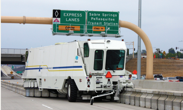
QuickChange Moveable Barrier: Enables real-time reconfiguration and improved safety.
