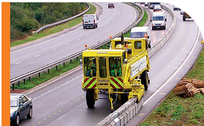
During construction, the Road Zipper system can help with off-peak lane closures or traffic crossovers ensuring positive protection for workers and motorists.
