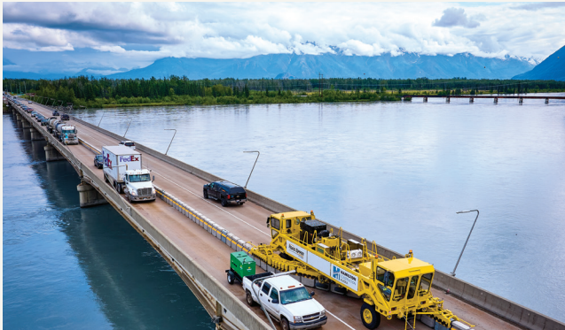
The Road Zipper Machine: Moves barriers for managed lanes, bridges, and construction.
