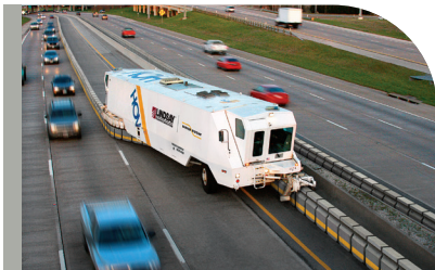
The Road Zipper System improves traffic flow, and safeguards work crews and motorists.
