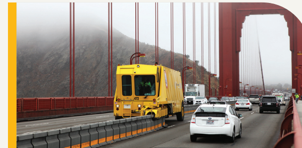
GOLDEN GATE BRIDGE / SAN FRANCISCO, CA Reversible Road Zipper managed lane (2.2 mile long) operational since 2015.
