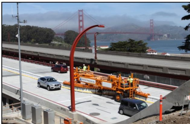
**QuickChange® Moveable Barrier reconfiguring the roadway under traffic to reduce congestion**
