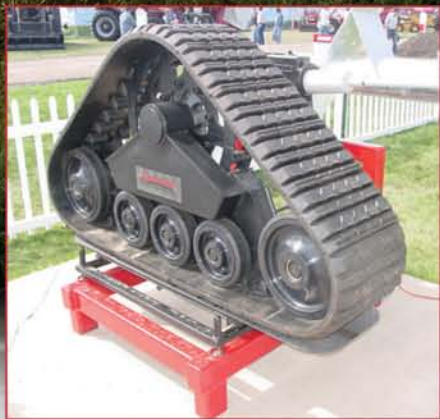
Lindsay's Z--Trax exchanges a pivot tower's tires with a rubber track. (Midwest Producer/Terry Anderson)
